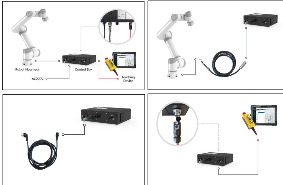
Chart 1.6-1 Wiring Panel of Control Box
